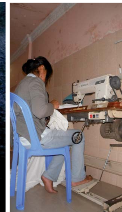
Foot powered sewing machine
